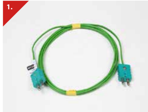
1. Compensating cable link cables To link controller/programmer thermocouple input to the recorder input. Stork reference & description: 34013 - 3m 'jumper' compensating lead fitted with two type K thermocouple plugs
