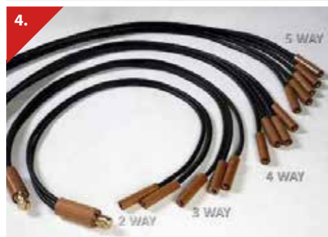
4. Splitter cables For use with triple cable sets. Splitters are used where the operator needs to connect multiple heating elements, in parallel, to triple cable sets to enable the control of multiple heating elements. This enables the heating elements to be grouped to a single control output from a heat treatment unit to allow accurate zonal temperature control. Stork reference & description: 32001 2 Way splitter 32002 3 Way splitter 32003 4 Way splitter 32004 5 Way splitter
