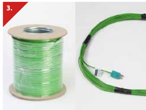
3. Thermocouple compensating cable Suitable for use with type K thermocouples where monitoring thermocouples, in addition to the control thermocouples, are required for temperature monitoring purposes. Available in 30m lengths complete with type K thermocouple plug and socket or in 100m rolls without plug and socket (plugs and sockets can be supplied separately as required). Stork reference & description: 34000 - 30m compensating cable c/w type K thermocouple plug and socket 504-062 - 100m roll of compensating cable without thermocouple plug or socket
