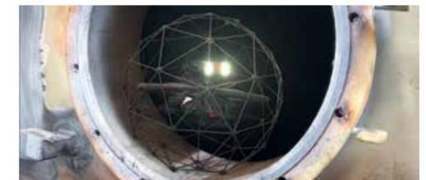
Elios drone inspecting a confined space.
