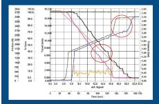
At first glance, the erratic opening and closing of the valve (black and pink lines) does indeed appear to be due to friction (the yellow line) caused by, for example, the gland packing. However, the lines circled in the top right corner, which represent the drive pressure, indicate a leak in the positioner. After repairing the positioner in-line, the analysis was repeated. The results given in the graph below show conclusively that the control valve is functioning properly again.
