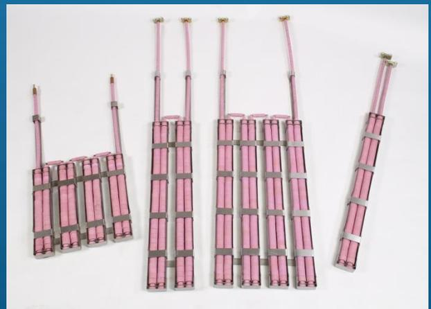
**Application – Internal bulk head heat treatment of vessel seams. (see illustration right)**
