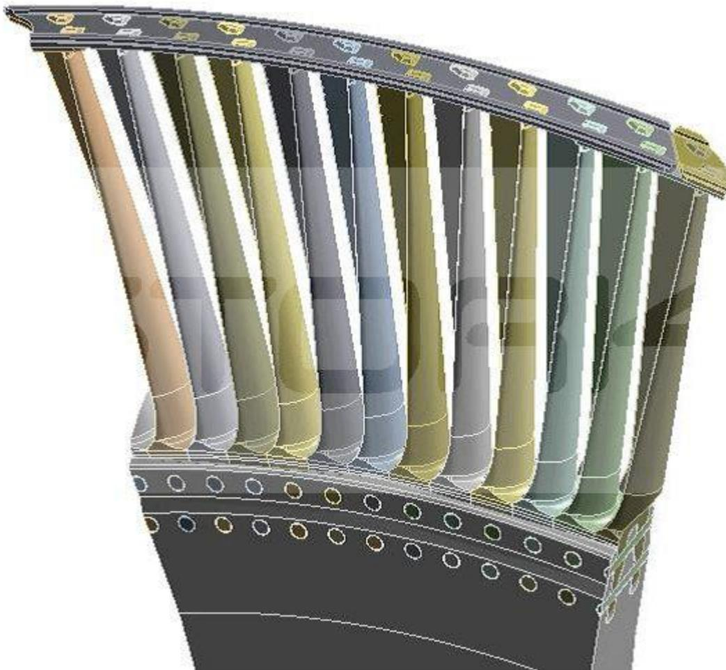
LP4 Blade Assembly with Shroud & Wheel
