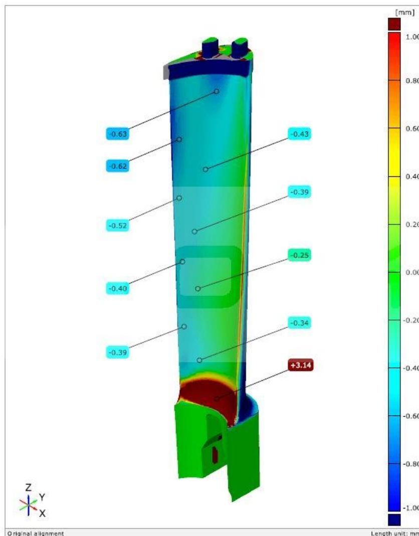
Example of CAD model dimensional checks
