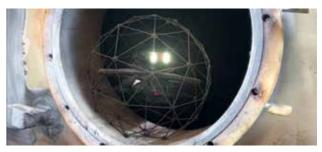
Elios drone inspecting a confined space.
