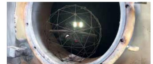
Elios drone inspecting a confined space.
