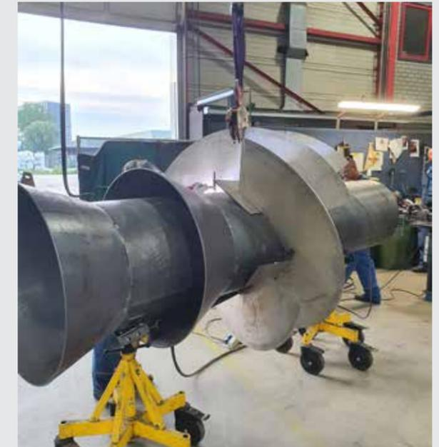
The project team decided that the best option would be to cut away the affected parts with a cobot \*) and called in the help of specialist Wecobot to get it done. A test setup was built in the Netherlands and was used as an online demonstration to explain the plan of approach to the technicians at Sakhalin. The true-to-life mock-up combined with the Stork technicians' specialist knowledge convinced the Russian client. That meant we had a GO. But under a very tight schedule.
