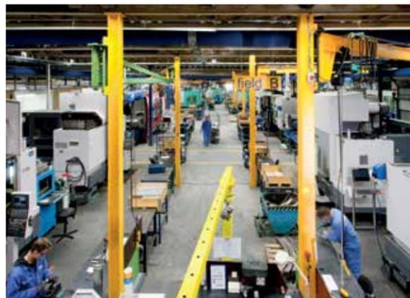
Stork Turbo Blading is the newest member of the Dutch Innovation Cluster Drachten. Turbo Blading uses technologies such as 3D reverse engineering to reproduce turbine engine blades. This advanced technology makes the production of comparable components possible, and redesign helps to improve the original parts.
