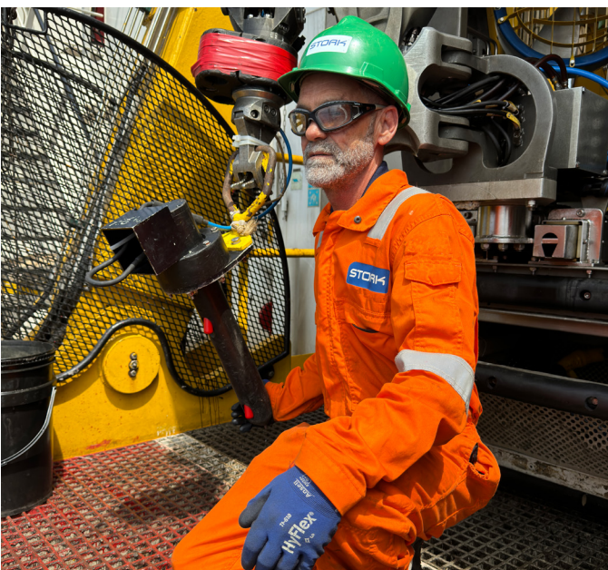
Stork personnel installing a CP probe mounted onto a ROV's multi-functional arm.
