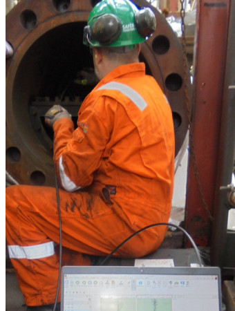
Photo: Remote Field Testing
